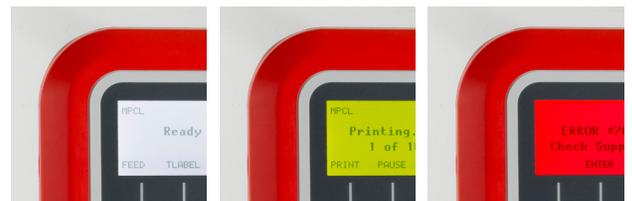
Three-color backlit display provides instant visual identification of printer status.
